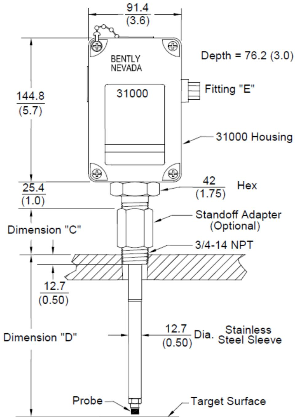
**Figure 1: Dimensions for 31000 and 32000 Proximity Probe Housings**
